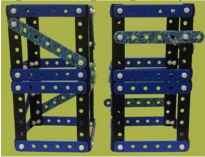
*Figure 1b: Low Alignability condition: unstable model on left, stable (braced) model on right, showing the two counterbalanced versions*
